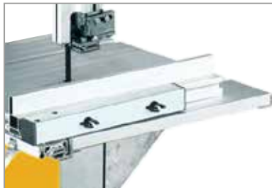
Tilting table up to 45° goniometer included
