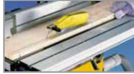
Circular saw \phi 200 mm with 45° inclinable rip fence Sierra circular \phi 200 mm con guía inclinable hasta 45°
