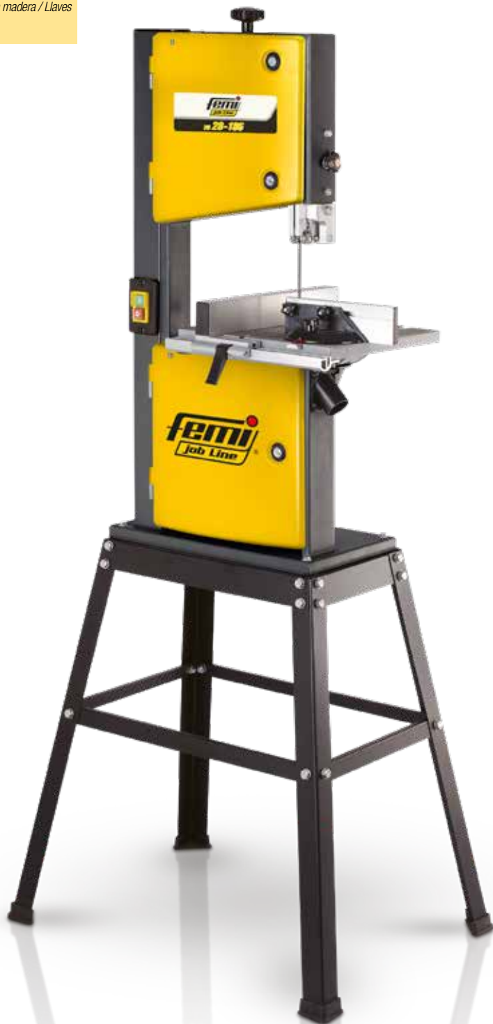
Aluminium tilting table up to 45°, goniometer include
